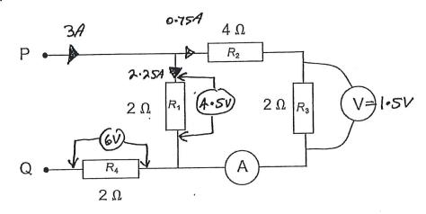
(a) Show that the total resistance between terminals P and Q is  $3.50\Omega$ .
