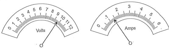
Determine the resistance R of the fuse wire.
